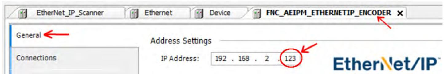
Or delete the device and “Scan for Device” again, this will automatically finds the scanned encoder’s IP Address.
