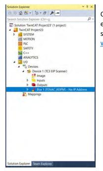
On the left side again right click on Device 1(TC3 EIP Scanner) and add new item to add encoder slave device from our eds file. Find FENAC\_AEIPM device from there and select it and click OK to add it. If you don't have the EDS file you can download it from <a href="http://www.fenac.com.tr">www.fenac.com.tr</a>.
