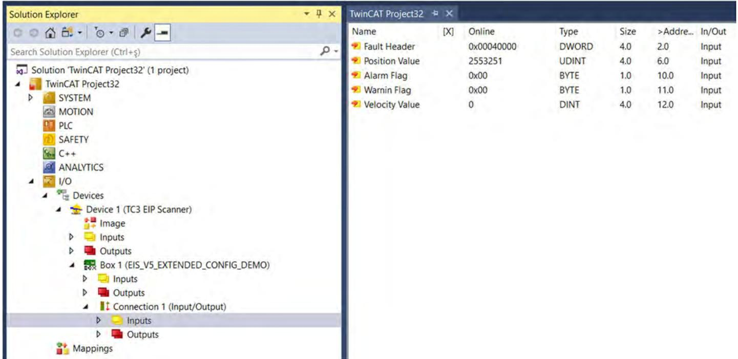
Here you can see the position value and Velocity Value changing when you turn the encoder shaft. These are the Process Data and it updates cyclically.
