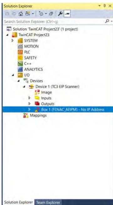
On the left side again right click on Device 1(TC3 EIP Scanner) and add new item to add encoder slave device from our eds file. Find FENAC\_AEIPM device from there and select it and click OK to add it. If you don't have the EDS file you can download it from [www.fenac.com.tr](http://www.fenac.com.tr).
