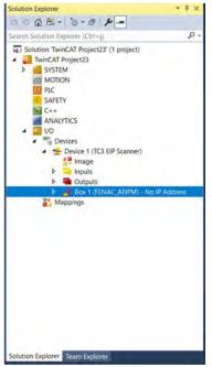
On the left side again right click on Device 1(TC3 EIP Scanner) and add new item to add encoder slave device from our eds file. Find FENAC\_AEIPM device from there and select it and click OK to add it. If you don't have the EDS file you can download it from <a href="https://www.fenac.com.tr">www.fenac.com.tr</a>.
