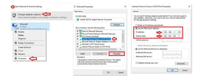
7) Open RSLinc Classic Application. Connect you PLC's usb cable (or ethernet) Under the USB section right click and select "Module Configuration". Under the "Port Configuration" tab, Set Port for A1 or A2 then set "Manually configure IP settings" and enter the value below in the image.
