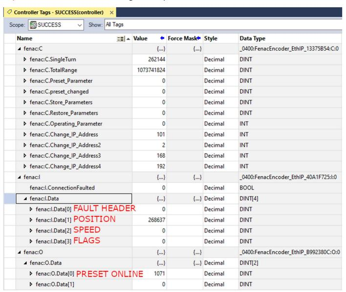
12) We need to change the status and Go Offline to be able to configure the encoder device. Most of the time, single turn value and total turn value are changing in encoders. Lets change the SingleTurn and TotalRange parameters (to do this we also need to enable scaling option with setting Operating\_Parameter to 4) We also try to preset device from 50 (to do this we need to enable preset\_changed to 1). After that we need to Download this new configuration to out encoder device.
