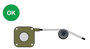
Pulling the rope straight is the most convenient option for use. This can be realised by using, however, a pulley.
