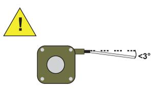
An angle of pulling direction up to 3° is possible, but not recommended. The lifetime may be reduced.
