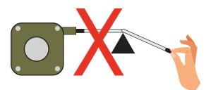
Don't pull the wire along of edges. The wires will be damaged.
