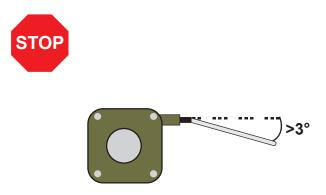
It is recommended to pull the wire straight. Pulling the wire at an angle higher than 3° will damage the wire and it will cause damage to the pull-back mechanism over time.
