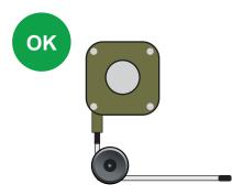
This mounting method should be preferred for any environment where humidity or dust is expected.
