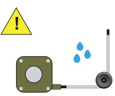
Horizontal mounting is possible if there is no risk of icing on the rope. If possible, the inlet should be mounted downside.
