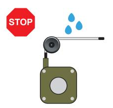
Complete sealing is not possible due to the structure of the wire. For this reason, the wire inlet should be mounted vertically in order to prevent the water from flowing along the wire and escaping into the wire unit.
