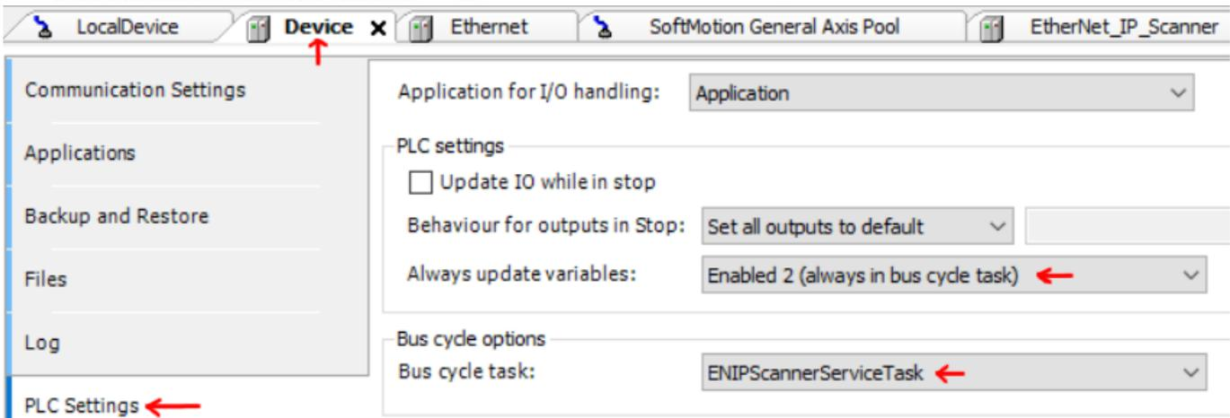
Finally under the Device tab click on PLC Settings and configure below settings.
