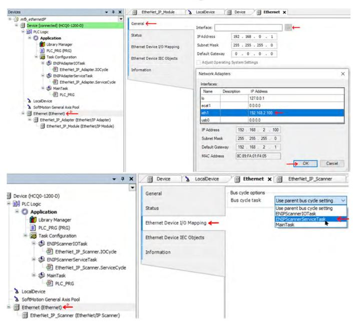
Finally under the Device tab click on PLC Settings and set below settings.
