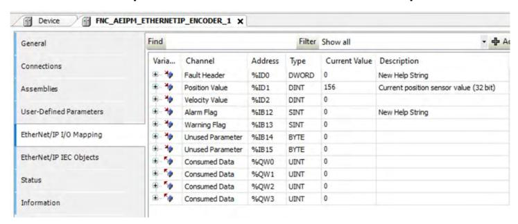
Here in this Ethernet/IP I/O Mapping page you can see the proccess datas like Position Value and Velocity value.
