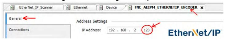
Or delete the device and "Scan for Device" again, this will automatically finds the scanned encoder's IP Address.
