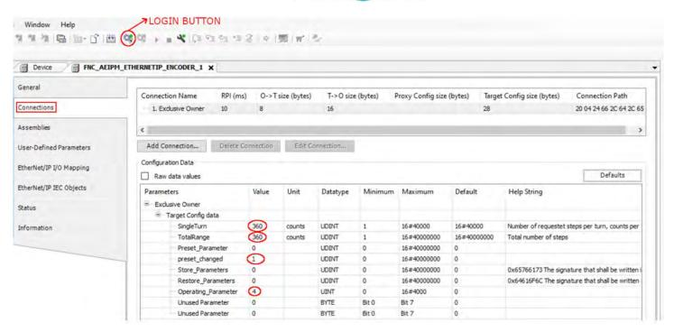
You can configure the parameters like "SingleTurn", "TotalRange", "Preset\_Parameter", "preset\_changed" and "Operating\_Parameter" here in this Connection page. After that you should click on "Login" button to set this parameters. Then start button to start operations.
