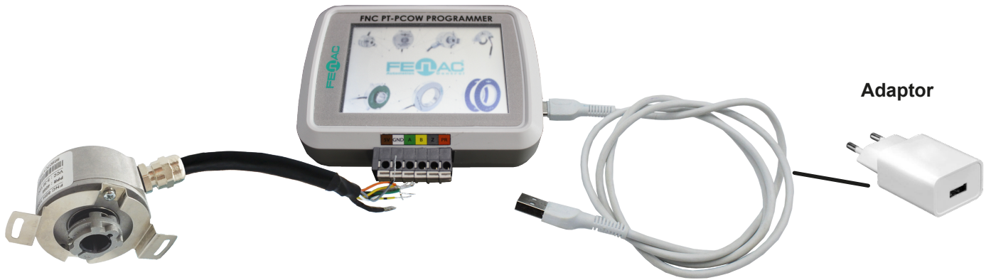
Programming Device Cable - Connected to Adaptor
