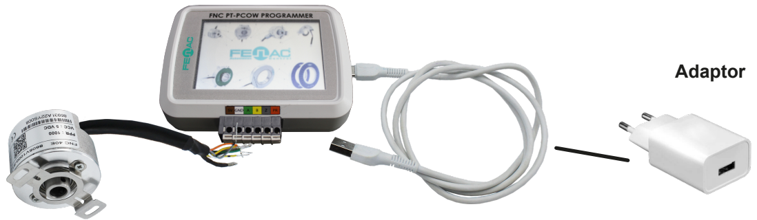
Programming Device Cable - Connected to Adaptor
